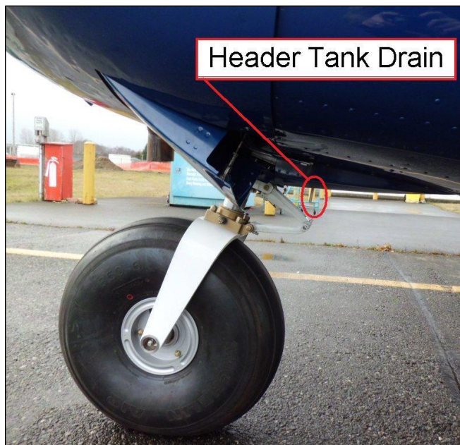
Figure 1-37 Header Tank Drain
