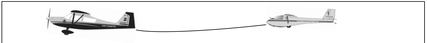
Figure 7-2 Glider 3 to 5 feet higher than tow plane
