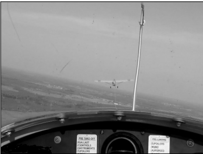
Figure 7-9 Correct Turn Position
