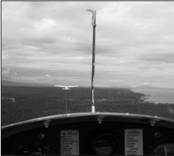
Figure 7-6 Tow Plane Wings on Horizon
